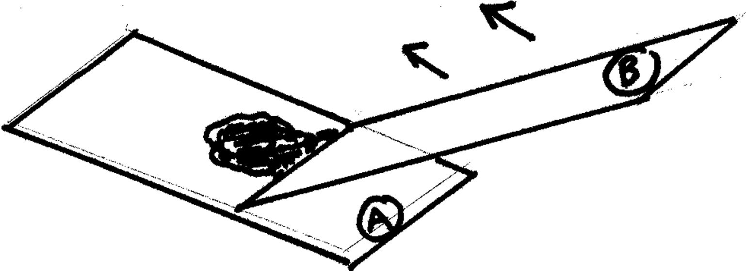
**Fig 9. Touch the lower edge of slide (B) on another slide (C) to drop the spicules**
