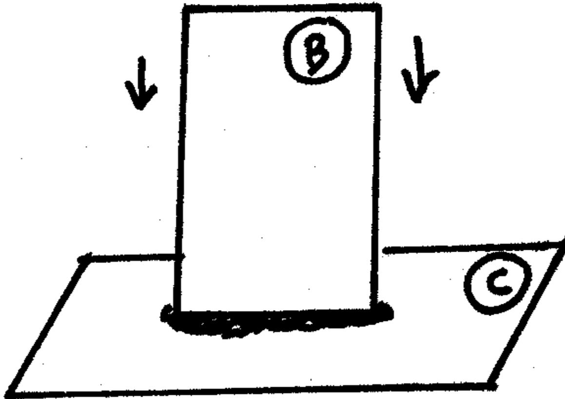
**Fig 10. Put (B) flat on (C), sliding (B) on (C) without much pressure**
